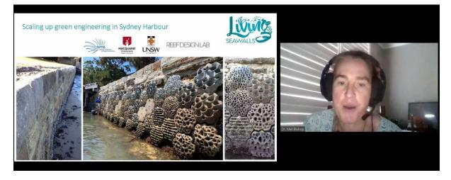
The overall intention is to replicate the effects that are created by rocky shorelines with tidal movements. In most cases, but not all, new seawalls are vertical, smooth or sloped at 45 degrees. The standout exception are the manmade retaining walls at Barangaroo.
