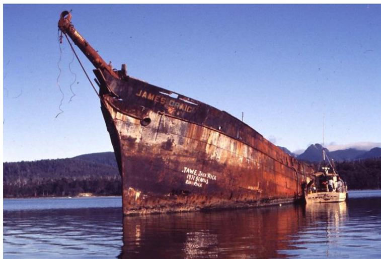
The first task was to patch the holes in the hull. This required Alan and several steel fabricators to spend three weeks camped on board the wreck, with only a tarp for shelter, in appalling weather conditions whilst they made repairs in order to tow her to Hobart. And this was only stage one!
